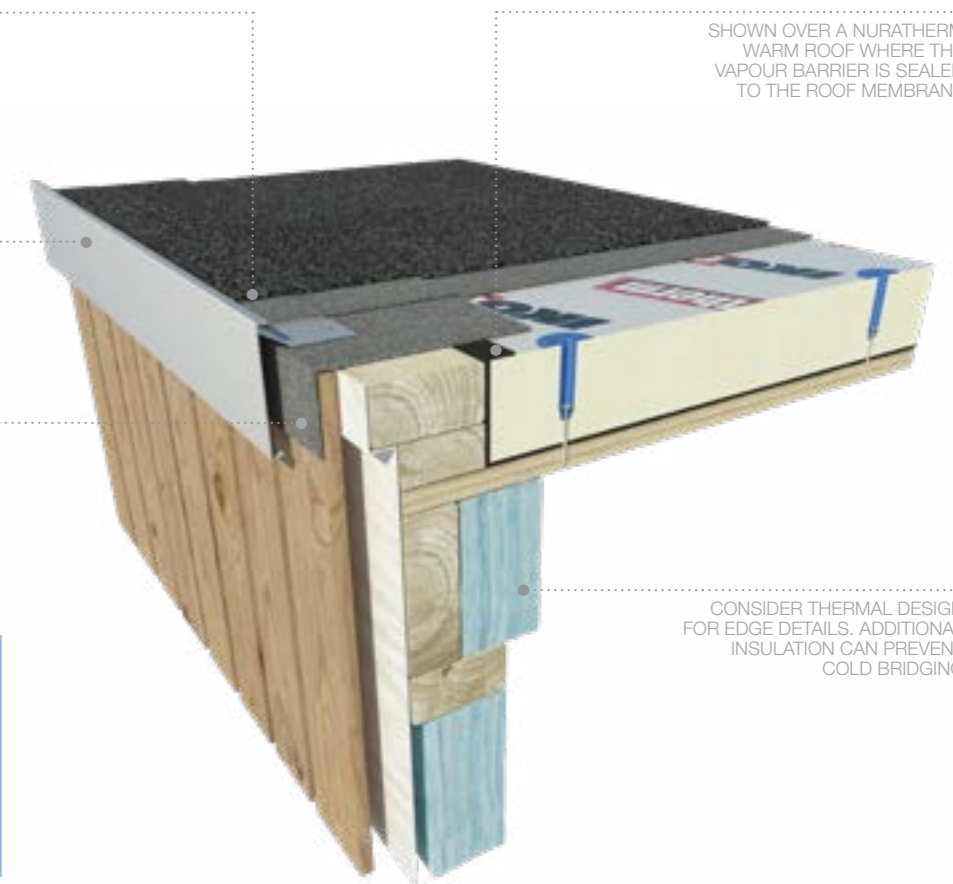
» Figure 17: NURATRIM. MECHANICALLY FIXED EDGING SYSTEM FOR RESISTING DYNAMIC WIND FORCES. DETAIL SHOWN WITH A NURATHERM WARM ROOF
